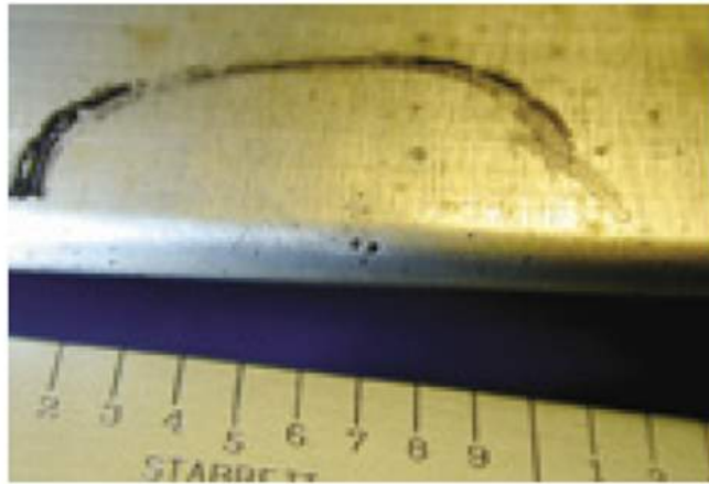
Qualitative comparison between actual and simulated eroded blade (pressure side)
