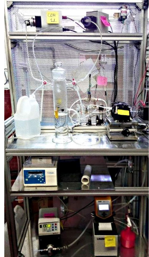
DMFC3. Test bench for small power size stack (< 380 W) characterization (VI curve, cross-over measurement).
