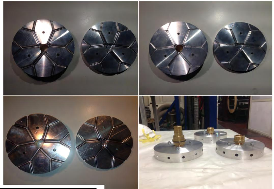
**“Constructal” heat exchangers:** theoretical analysis, validation of design concept & testing of 3 prototypes.
