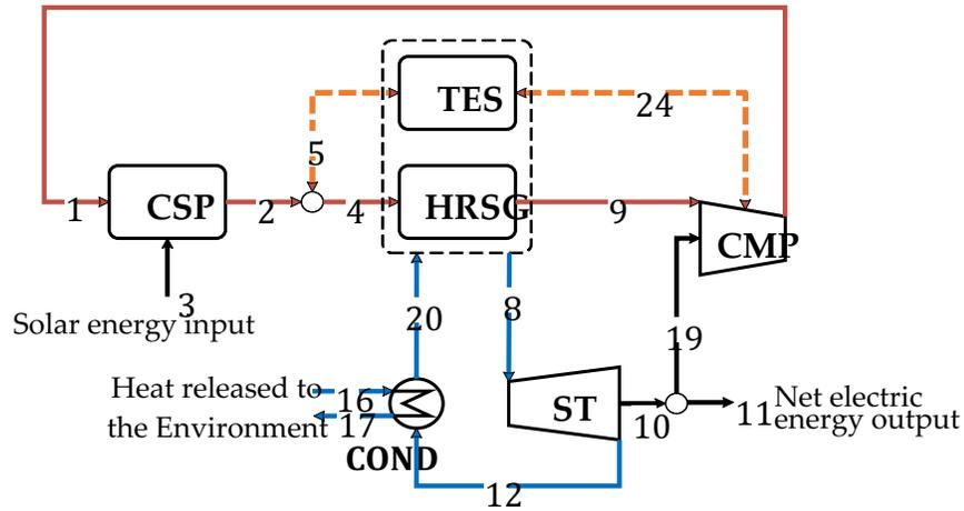
The Julich (J-CSP) CSP plant with thermal energy storage has been compared with a Hybrid plant (H-CSP) using air as working fluid
