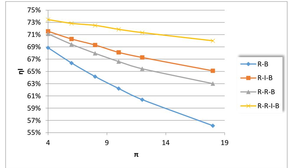
Comparison of thermal efficiency of Brayton cycles with different configurations
