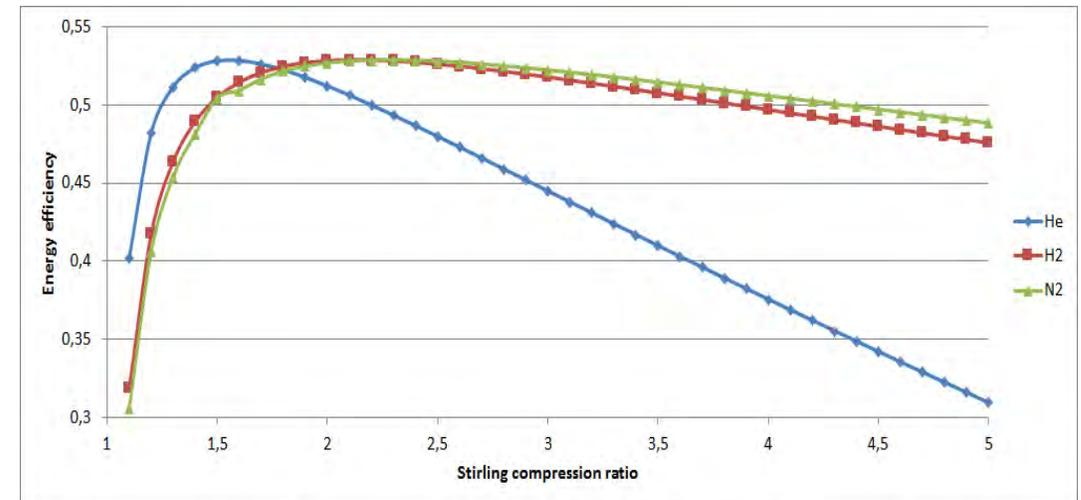
Stirling cycle thermal efficiency comparison for different working fluids ( $T_H=1500K$ ,  $T_L=200K$ ,  $\epsilon_r=0.85$ )
