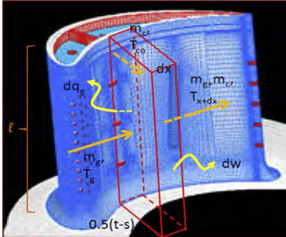
At a given PR, a **maximum in thermal efficiency** is likely to be reached below stoichiometric conditions, imposed by the **large amounts of cooling air** required
